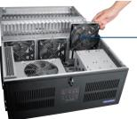
Intelligent System Module Two 5.25" and one 3.5" disk drive bays
