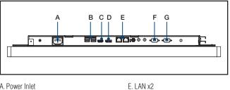
A. Power Inlet B. USB3.2 x 4 C. USB Type C D. HDMI
