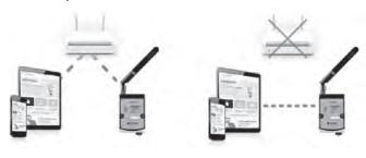
Data logger can push the data to file-based cloud services like Dropbox using pre-configured criteria. With RESTful API, the data can also been pushed to a private cloud server in the format of JSON. Users can setup their private cloud server using the provided RESTful API and their own platform.
