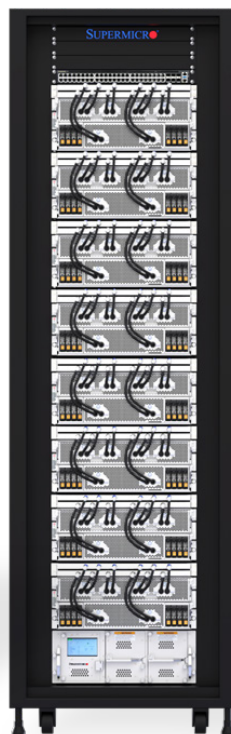
4U Supermicro NVIDIA HGX 8-GPU Systems
